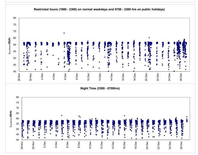
After checking with Contractor of HY/2009/19, on 15 December 2015, concreting was undertaken by Contract HY/2009/19 while steel bar cutting works for Hong Kong Electric Centre was conducted at the roof top by non-CWB Contractor immediately next to the noise monitoring station. In view of the mitigation measures implemented and the non-CWB works conducted next to the monitoring station as major noise contribution, the exceedance was considered as non-Project related.
